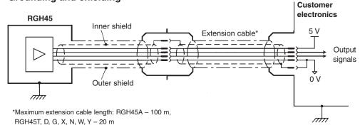
**IMPORTANT:** The outer shield should be connected to the machine earth (Field Ground). The inner shield should be connected to 0 V at receiving electronics only. Care should be taken to ensure that the inner and outer shields are insulated from each other. If the inner and outer shields are connected together, this will cause a short between 0 V and earth, which could cause electrical noise issues.
