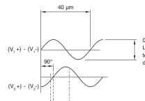
0.7 - 1.2 Vpp with green LED indication and 120R termination when signal is differentially received
