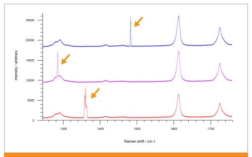
Figure 1. Different examples of CR artefacts in a Raman image. The sharp and intense nature of the features make them highly invasive to our Raman spectra. Top - typical CR on spectral baseline; middle - CR on top of Raman band; bottom - broader and structured CR feature.
