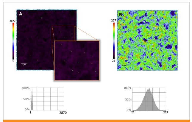
Figure 2. Raman images showing the intensity variation of the C=C peaks across the resin sample: (A) without CRR pre-processing; and (B) with CRR pre-processing. The Raman image with CRR processing shows greater sensitivity to changes in C=C intensity. The respective histograms show the distribution of intensity values in both cases and how CRs can significantly distort the Raman image.
