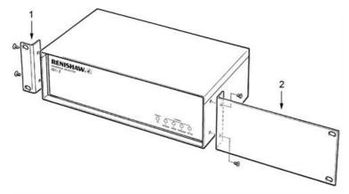
$The \ rack \ mounting \ bracket \ kit \ is \ part \ number \ A-1018-0124. \ The \ blanking \ panel \ kit \ is \ part \ number \ A-1018-0123.$
