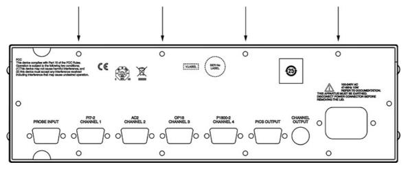
• Then remove the retaining screw on each side of the box:
