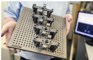
Multiple part set-up increases throughput on CMM.
