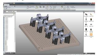
FixtureBuilder screen with Tritech components.
